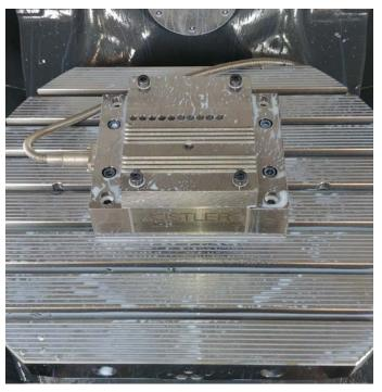
Detailed top view of the 9119AA dynamometer from Kistler, which precisely measures forces and moments in all three spatial directions.
